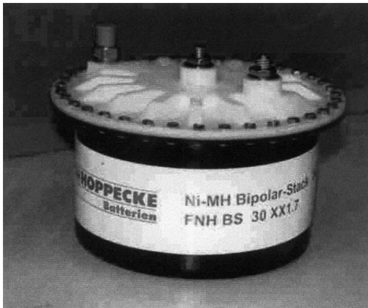
Fig. 2. Laboratory bipolar stack. 36 V, 1.7 Ah.
